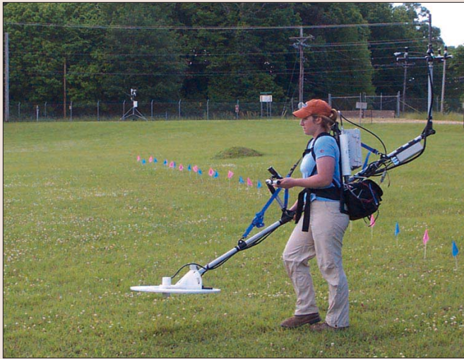
Figure 6. Field demonstration of the ERDC hand-held dual-sensor TFM-FDEM system, with integrated Arc Second six-degree of freedom positioning system, at the ERDC UXO test site, April 2005.
