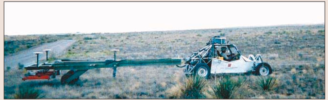
Figure 9. The VSEMS (a towed dual-sensor array system).
